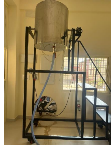
ICAR-IIHR designed grain boiler
