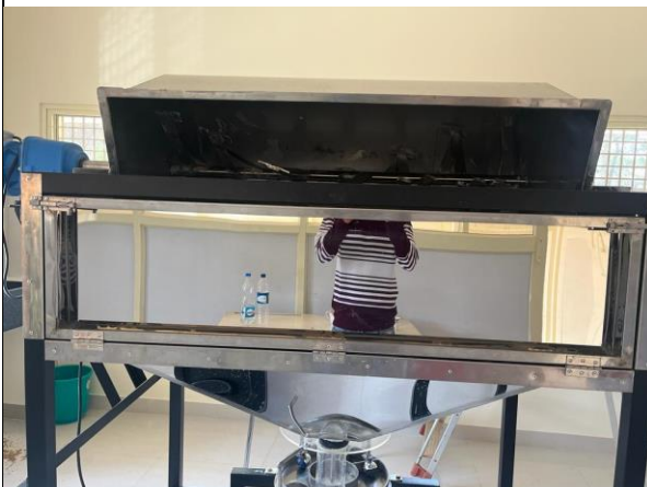
ICAR-IIHR designed grain mixer cum filling machine
